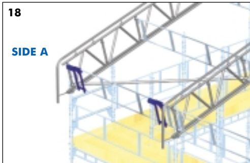
Figure 18 Fit pair of Eaves Roller Brackets to end Lacing Frames at each side of roof.
