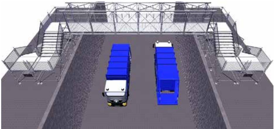
15m HAKI Bridge System
