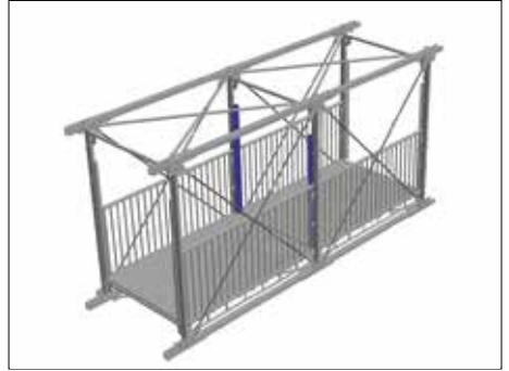
2. Install H-Track Units in the middle bays.
