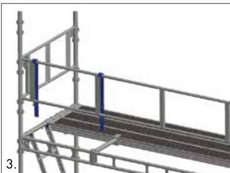
3. Install 2 double beam riders onto the Guard frame.
