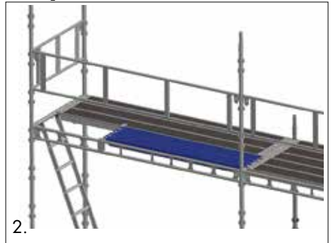
2. Install 2x1964 steel decks over the transom and board to ledger bracket. Install the ladder over the transom.
