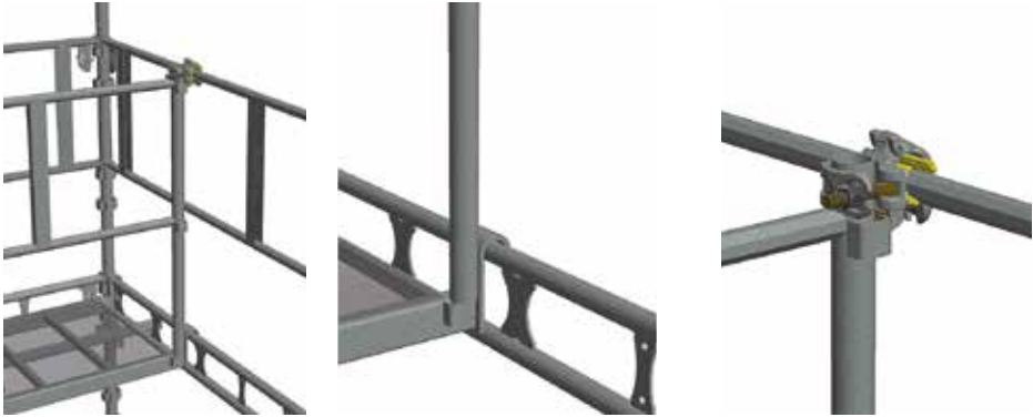
HAKI MK1 – P-Frame before 2007. Addition of Adapter 35 and Double Coupler
